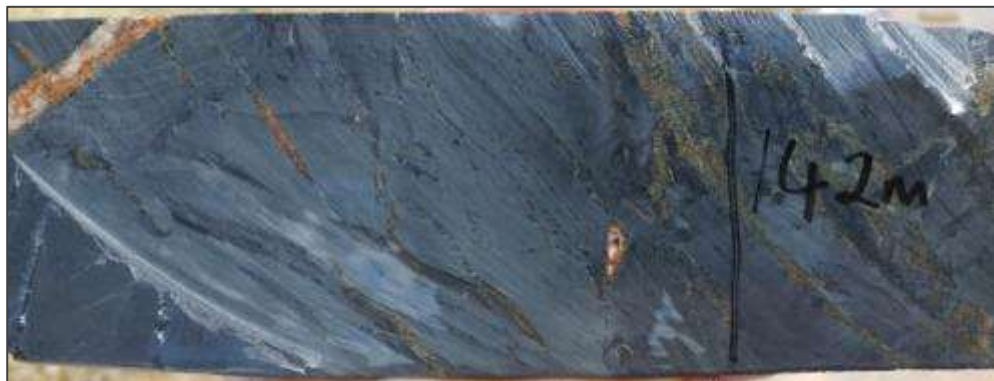
Figure 12-3 Veinlet-related pyrite-chalcopyrite mineralisation at 142 m in SHAK0007
