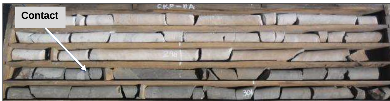
Figure 7-15 Chilled contact between dolerite and partly bleached Dwyka siltstone (first three rows) in CKP-8A
