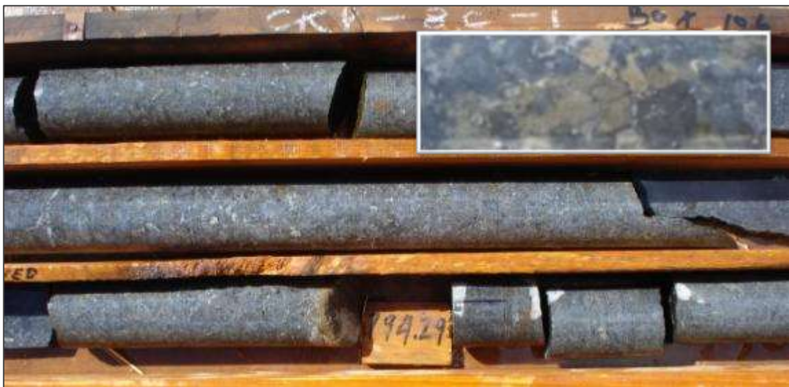
Figure 7-16 Medium- to coarse-grained mela-gabbro and pyroxenite (inset) of the Tshane Complex in CKP-8C-1
