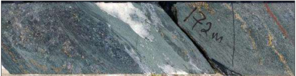
Figure 12-1 Concentrations of chalcopyrite ± pyrite along foliation planes within a shear zone developed in gabbro in SHAK0004
