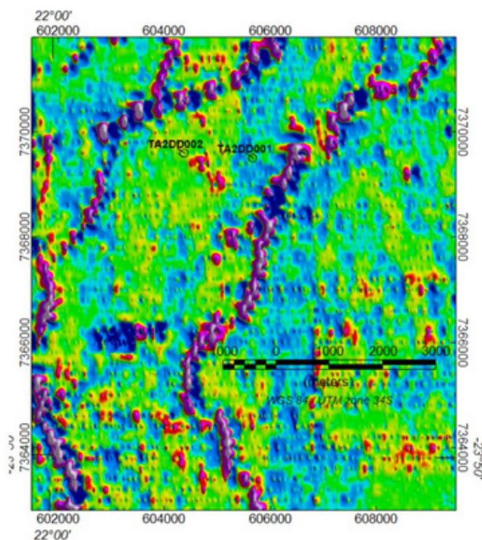
Figure 5. Anomalies removed from original measured ground magnetic data using non-linear filtering.
