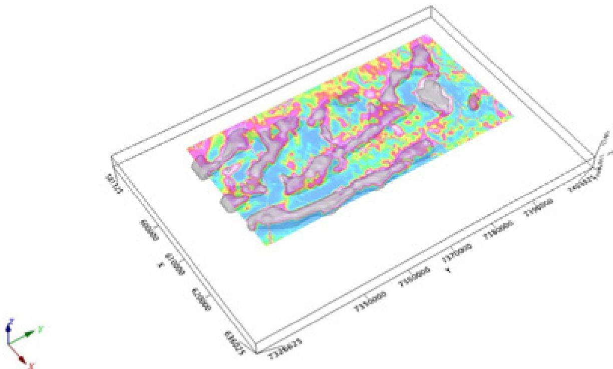
*Figure 2. 3D magSus model for deep (Proterozoic) magnetic sources derived from airborne magnetic data. Correlation between magSus bodies and magnetic anomalies is very good.*
