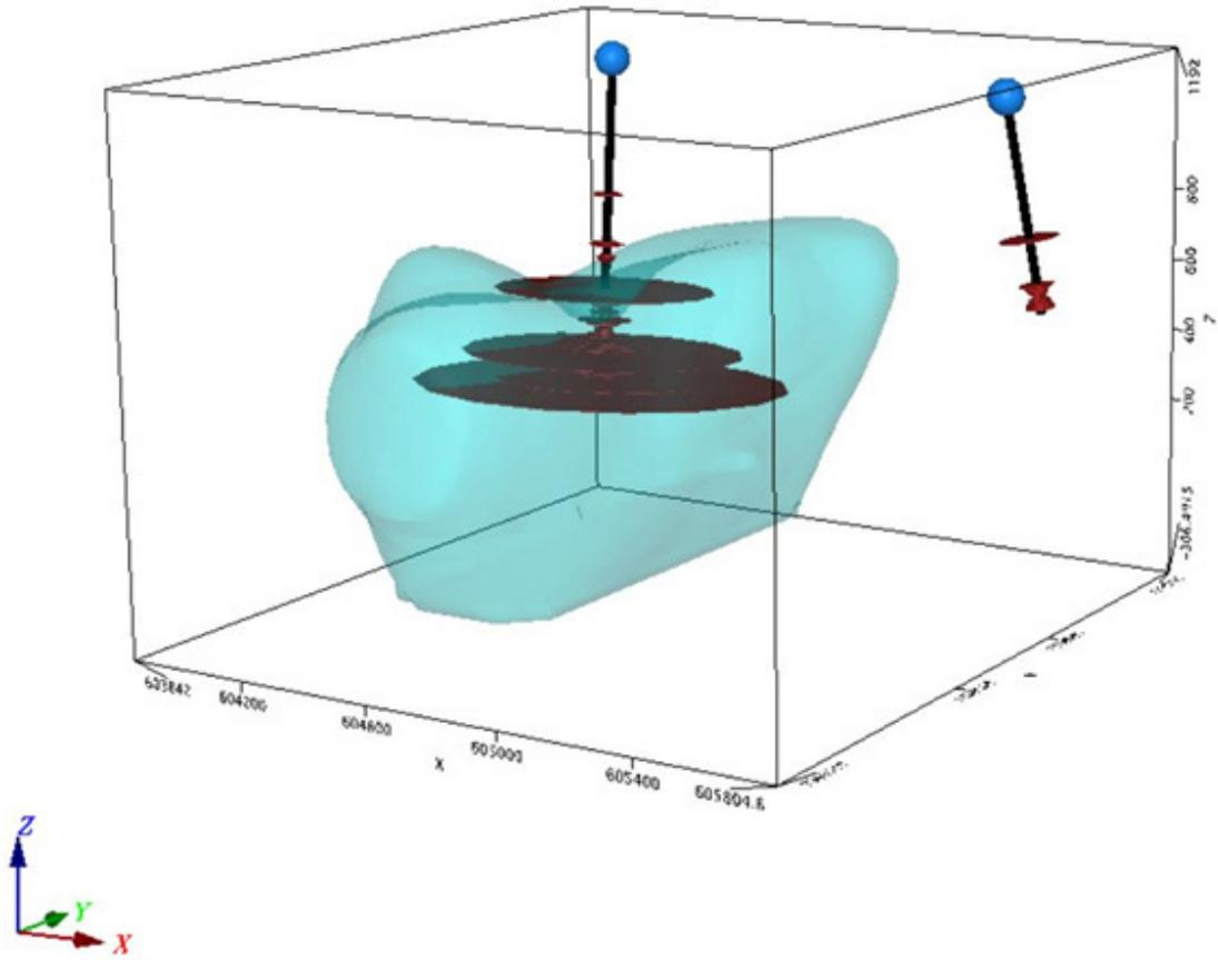
Figure 7. Perspective view from the SE of magsus iso-surface  $5.5 \times 10^{-3}$ SI units.
