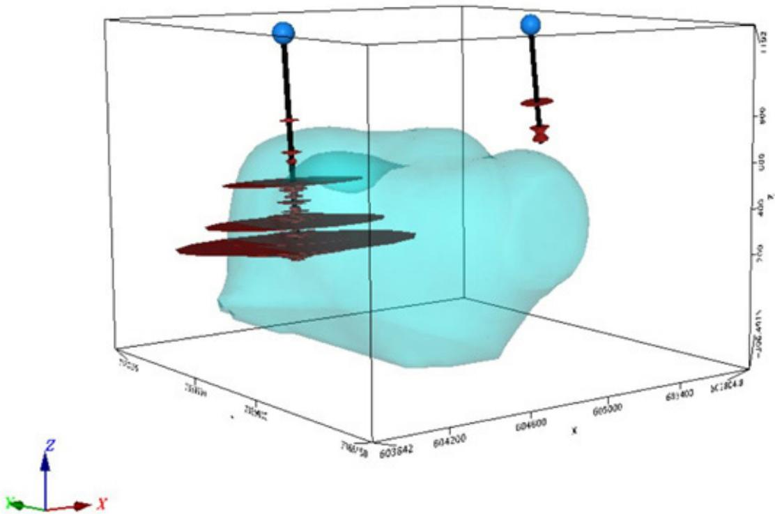
Figure 8. Perspective view from the SW of magsus iso-surface  $5.5 \times 10^{-3}$ SI units.
