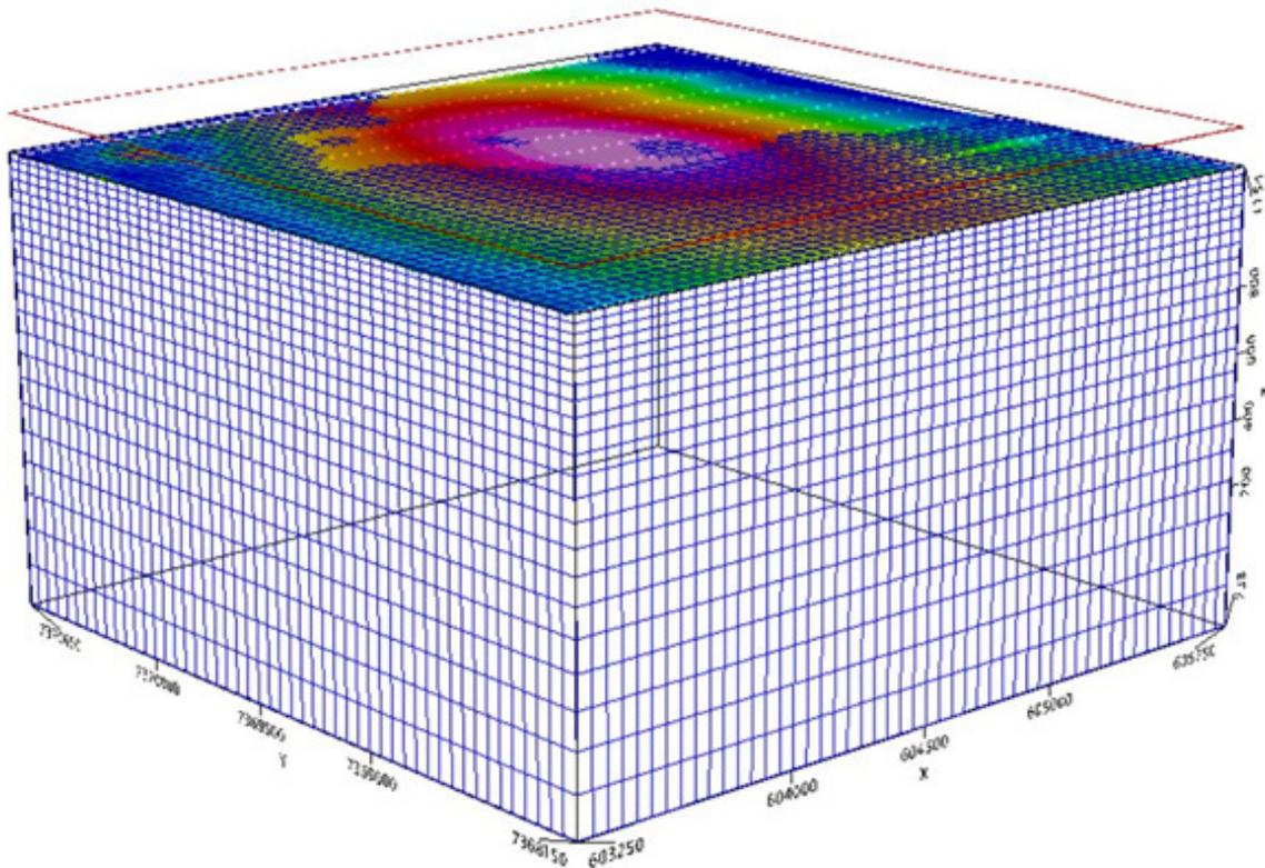
Figure 6. 3D mesh used for inversion of ground magnetic data – 50m resolution.
