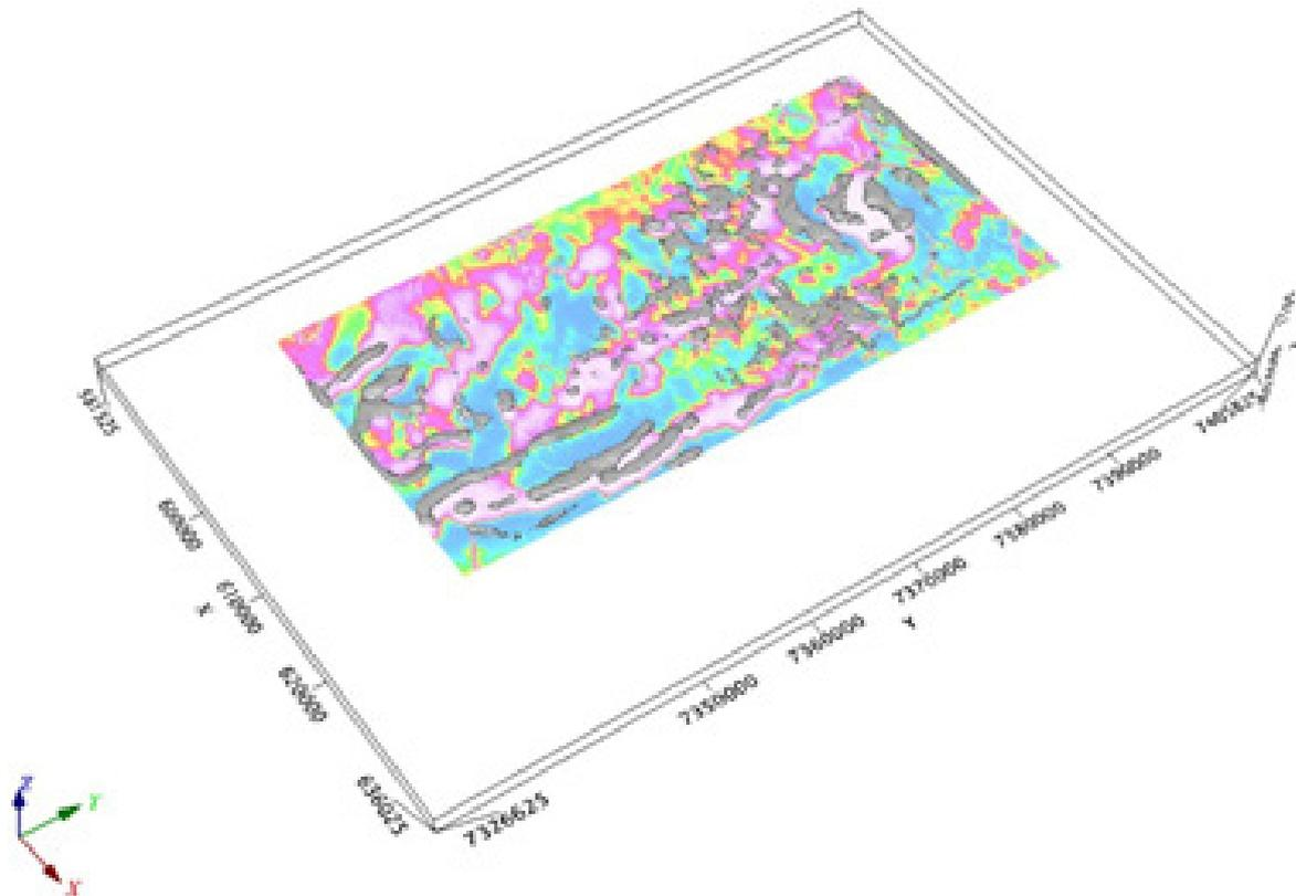
*Figure 1. 3D magSus model for shallow (karoo) magnetic sources derived from airborne magnetic data. Correlation between magSus bodies and magnetic anomalies is sub-optimal.*
